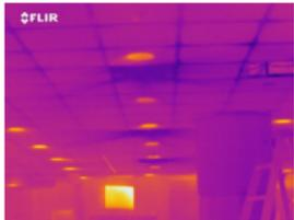
Two types of energy loss can occur within a building envelope. The first type of loss is conduction. Conduction losses are most often due to missing/damaged or water-saturated insulation within the building wall and/or roof. Under proper weather and site conditions, our Infrared Building Envelope Surveys can detect and document evidence of energy loss or latent moisture within building sidewalls including EIFS clad structures.
