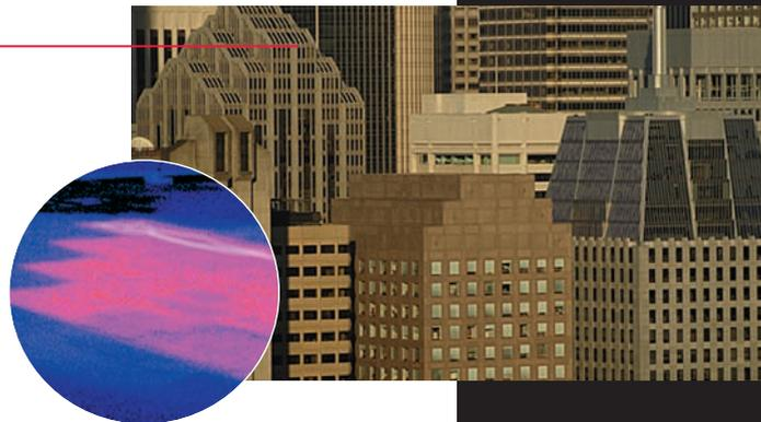
Thermogram shows warm area on flat roof caused by moisture infiltration into roofing system.
