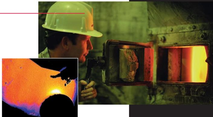
Thermogram shows hot spot on catalyst line caused by refractory failure.
